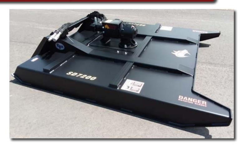
Standard duty models utilize all the same drive and blade carrier components as our tried and true heavy duty models at a more budget friendly cost. A lighter support structure, limited guarding, and removed chain curtains are some of the modifications made to provide a more economical cutter option.
