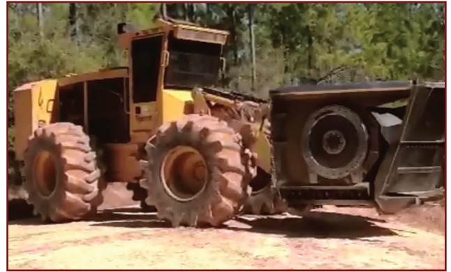
192A - Two hydraulic retractable wings adjust for transport and your environment*
